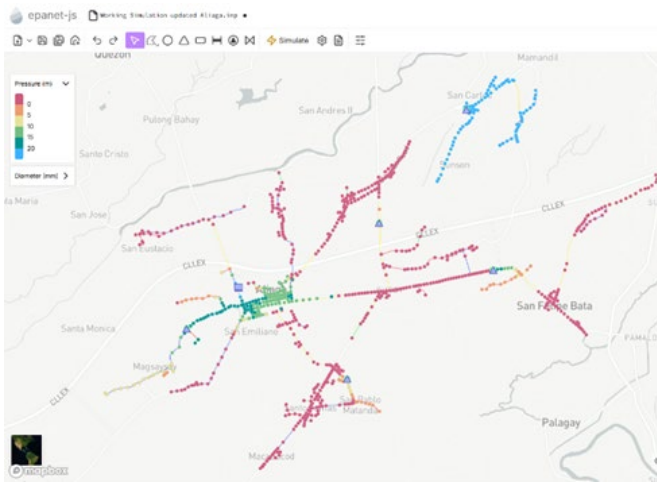
Figure 6: Nodal Pressure Distribution – 2035 Medium-term Projection
